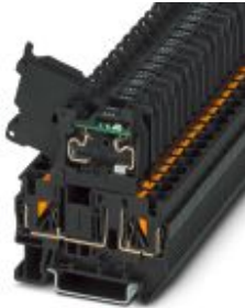
Lever-type fuse terminal block, black, for 5 x 20 mm G fuse inserts, with LED for 24 V AC/DC
