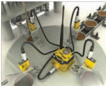
Wireless Monitoring of Rotary Table
