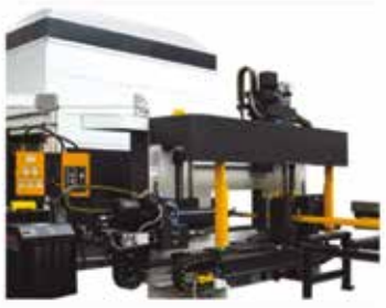
Beam drilling and sawing machines
