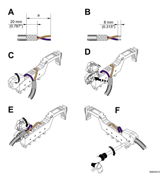
Figure 6 Connecting the shield via the shield connector
