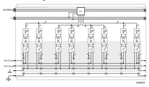
Figure 3 Internal wiring of the terminal points
