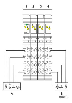
Figure 4 Typical actuator connections
