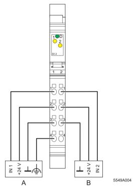
Figure 4 Typical sensor connections
