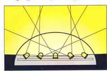
Patlite has created a revolutionary lighting design (patent pending) in which multiple LEDs project light across a broad peripheral area, ensuring equal intensity at the sides as well as the front. This design, with its side-projection technology, is a unique achievement in signal light design.
