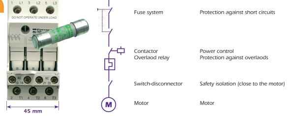
In a typical motor starter set-up the advantages to using a fuse rather than a circuit breaker are obvious: Cost savings on maintenance,
