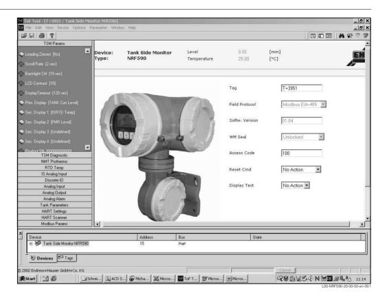
The Tank Side Monitor can also be operated via the "ToF Tool - Field Tool Package". This program supports commissioning, securing of data, signal analysis and documentation of the instruments. It is compatible with the following operating systems: Win95, Win98, WinNT4.0, Win2000 and Win XP.
