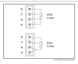
A spot RTD can be connected to the NRF 590 if the option is installed. For 4-wire connection, the RTD must be connected to the 4 available terminals marked D+, S+, S- and D-. For 3-wire connection, the RTD should be connected to the same 4 terminals. The terminals D- and S-should be connected together.
