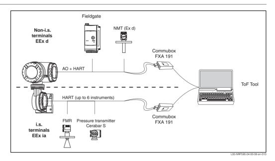
Up to 6 sensors can be connected in multidrop mode to the intrinsically safe HART loop. Typical process variables measured by the HART sensors are:
