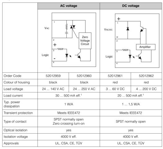
1) This upper limit of the load current is determined by the Tank Side Monitor.
