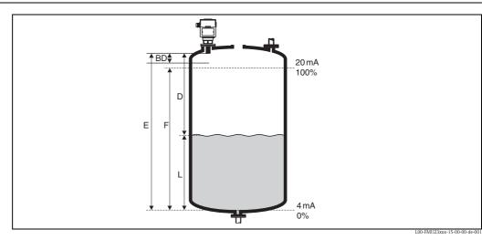
E: Empty distance; F: Span (full distance); D: Distance from sensor membrane - product surface; L: Level; BD: Blocking distance
