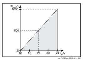
The maximum load  $(R_{\text{max}})$  depends on the supply voltage (U).
