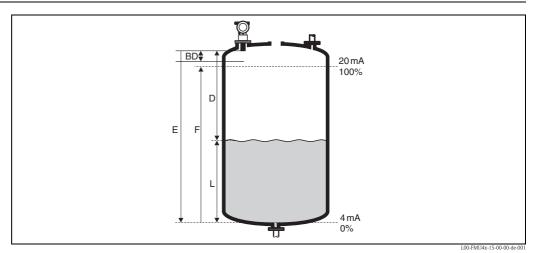
E: Empty distance; F: Span (full distance); D: Distance from sensor membrane – product surface; L: Level; BD: Blocking distance
