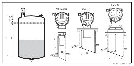
BD: blocking distance; SD: safety distance; E: empty calibration; F: full calibration (span); D: nozzle diameter; L: nozzle length
