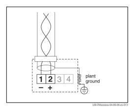
The digital communication signal is transmitted to the bus via a 2-wire connection. The bus also provides the auxiliary energy. Use 2-wire twisted pair cable with screen.
