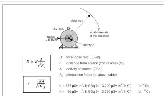
The control area is defined as that particular distance r from the source by which the local dose rate is attenuated to a value D when using an activity A.
