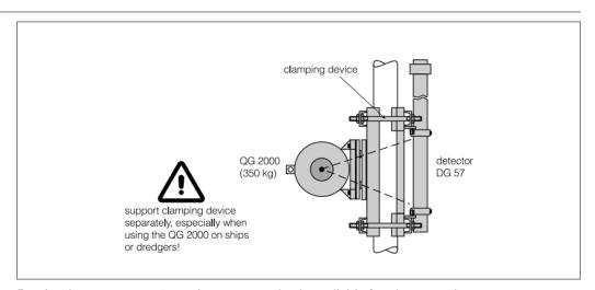
For density measurements, a clamp connection is available for pipe mounting.
