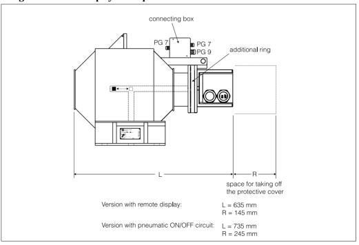
The standard design can be upgraded to the designs with remote display and pneumatic ON/ OFF circuit by a set.
