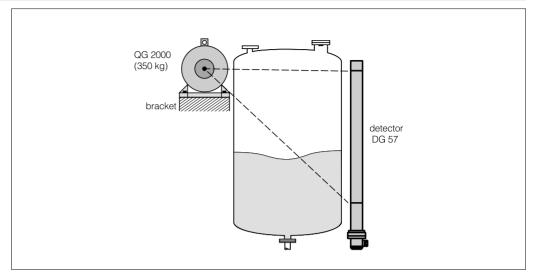
In order to ensure stable measurement and lasting radiation protection, the QG 2000 must be tightly screwed onto a rugged, low-vibration bracket that can withstand a weight of 350 kg under all operating conditions. Additional supports are generally required when mounting directly onto the vessel. A fastening for a crane on the QG 2000 is provided for transporting it.
