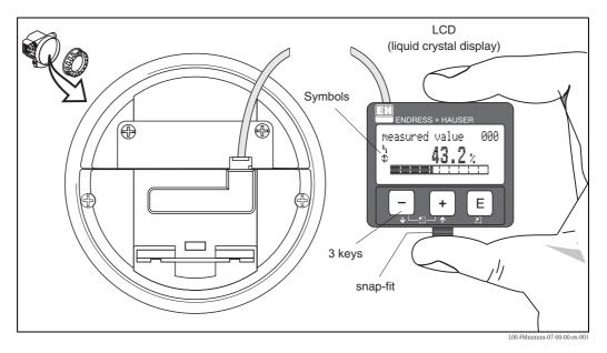
The VU331 LCD display can be removed to ease operation by simply pressing the snap-fit (see graphic above). It is connected to the device by means of a 500 mm cable.
