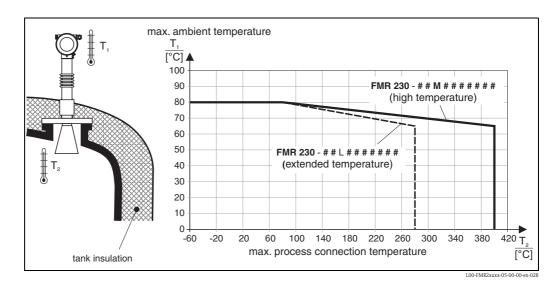
For process connection temperatures (T2) above  $80^{\circ}$  C, the allowed ambient temperature (T1) at the housing is reduced according to the above diagram.
