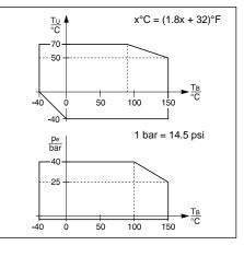
Top graph: Permissible values for ambient temperature  $T_u$  at housing are dependent on the operating temperature  $T_B$  in the tank Bottom graph: Permissible values for operating pressure  $p_e$ are dependent on the operating temperature  $T_B$  in the tank
