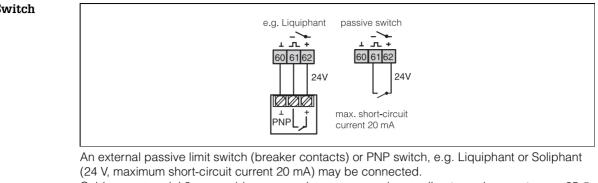
Cable: commercial 3-core cable, screened or unscreened according to environment, max. 25  $\Omega$  per core.
