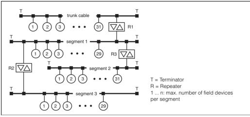
Several repeaters can be used to create a tree structure. The number of participants allowable per segment is reduced by one per repeater: the total number of participants is limited to 126 -(2x number of repeaters).
