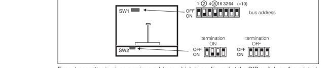
Every transmitter is given a unique address which is configured at the DIP-switch on the printed circuit board.
