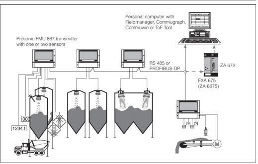
The measuring system comprises several transmitters Prosonic FMU 867. One or two sensors FDU 80 ... 86 may be operated on each transmitter. For special applications further instruments may be connected to each measuring point:
