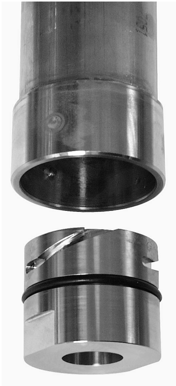
Measuring cell holder with bayonet lock
