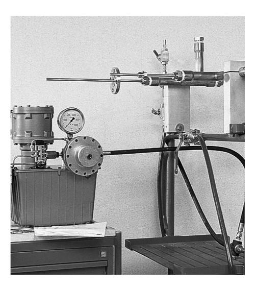
At E+H Temperature Production Centre, the total service approach is a standard....you can ask to a temperature supplier specialist! Our Temperature Production Centre specialists know your problems and are qualified to support you with hydrostatic test for thermowells.
