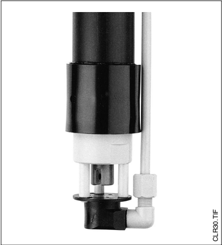
left: Spray head CLR 30 for Chemoclean cleaning system; can be retrofitted, no need to convert the assembly; material: PP
