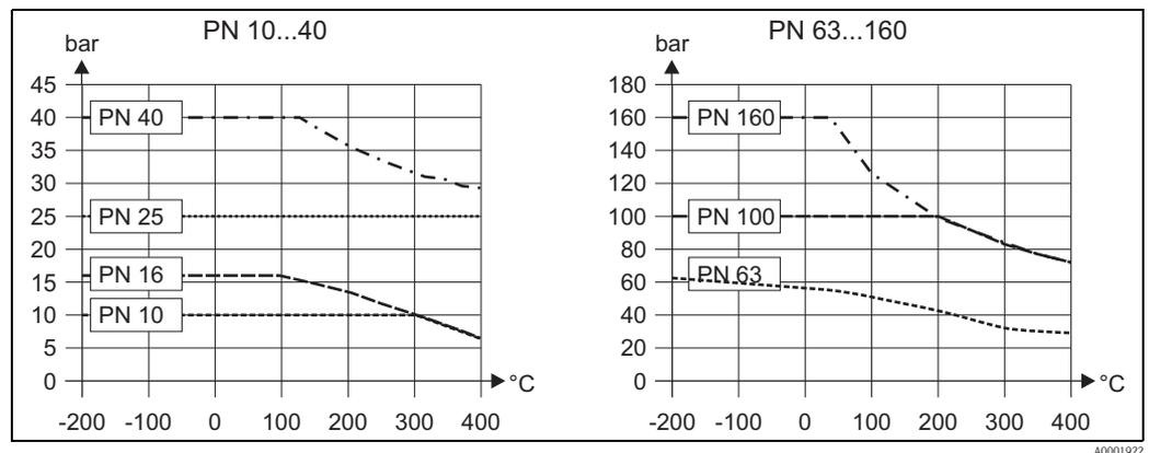
**Pressure-temperature curve according to ANSI B16.5 and JIS, stainless steel**
