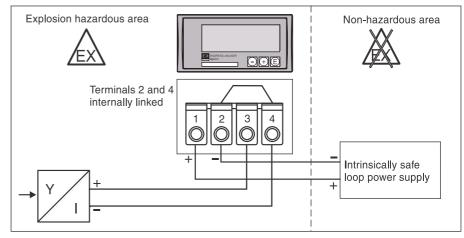
When using an Ex certified display it can be applied as a front end display in the non-explosion hazardous area.
