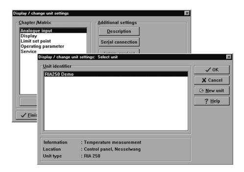
The RIA250 can be set up extremely easily using the built-in RS232 serial interface and the ReadWin®2000 PC software. Safe and secure setting up is made possible via on-line help text. ReadWin®2000 software package and interface cable are available as accessories.
