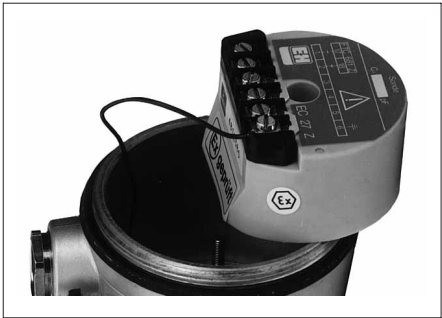
Connection of the electronic insert EC... in the probe housing
