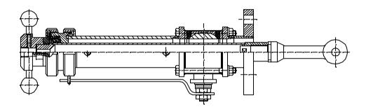
The manual retractable sensor holder for the measurement of inductive conductivity is fitted with a ball valve for separation from the process with 2" threading. Connection to the process by means of a flange of DN50/PN10 material in 1.4571. Immersion depth from beneath the flange 180 mm.
