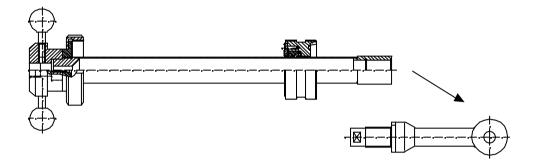
To extract the CLS50 sensor, loosen the cable clamp PG11 and then undo the sensor from its support. At this point pull out the cable being careful not to tear it.
