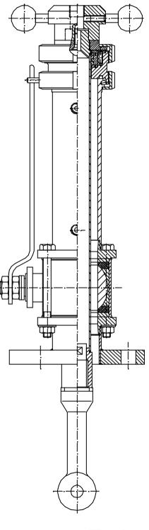
With this retractable assembly it is possible to extract the sensor by hand for simple maintenance or calibration, cutting off the process with pressures up to 3 bar (note 1).
