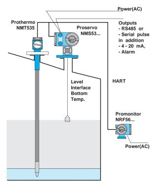
Promonitor is a tank side monitoring and control station for the Proservo series of intelligent tank gauges.
