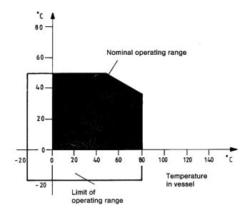
Fig. 3  $\triangle$  Permissible operating temperatures for the SOLIPHANT or LIQUIPHANT level limit switch with integrated relay module.
