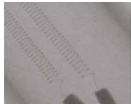
Wire spiral of a wire wound sensor with approx. 20 µm wire diameter
