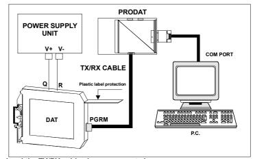
Warning: during these operations the device must always be powered and the TX/RX cable always connected. For information about DATESOFT refer to the software's user guide.
