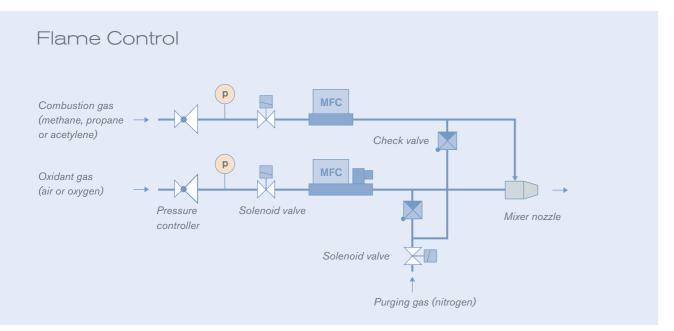
MFCs and MFMs are used to provide combustion gas and oxygen in precise ratios.
