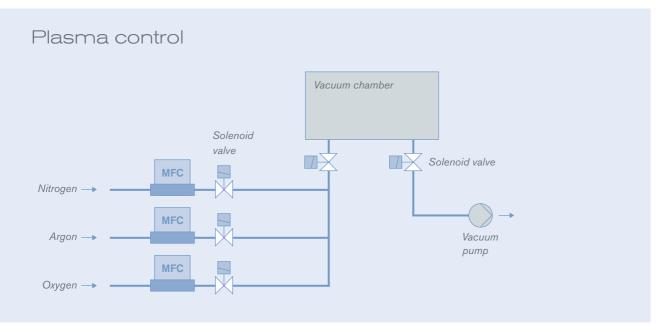
MFCs precisely dose gas and gas mixtures into a vacuum chamber and therefore enable products to be processed in a plasma atmosphere.
