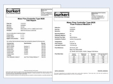
A calibration certificate is created for each MFM/ MFC after calibration. Two calibration certificates are provided for MFMs/MFCs supplied for the use of two gases or for devices with a wider measuring span.
