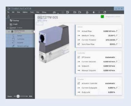
User interface of the Bürkert Communicator. The graphical programming interface (f(x)) is integrated into this software. The f(x) allows to program customized system control functions – e.g. for gas blending.
