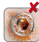
STAINLESS STEEL + NO STAINLESS STEEL = RUST
