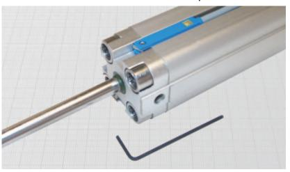
These sensors are completely electronic and detects the position of the magnetic ring inside a standard pneumatic cylinder with a T slot. The sensor remains completely recessed and thus mechanically protected. Main advantages of static output sensors are unlimited electric life, protection against short circuit and lines transient, high switching frequency and no bounces on switching edges. A yellow LED gives indication of the output status. Available with cable exit or connector M8x1.
